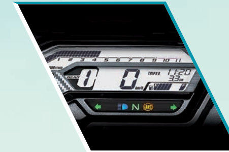
STREET-TECH DIGITAL METER With innovative displays like service due indicator and gear position indicator
