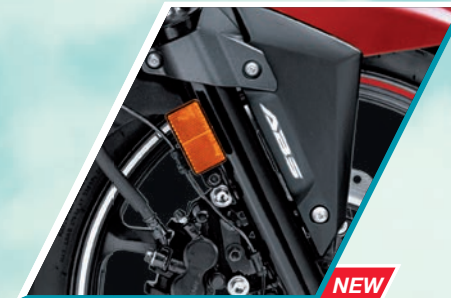
ABS WITH PETAL DISC BRAKE Prevents the front wheel from getting locked in case of sudden braking
